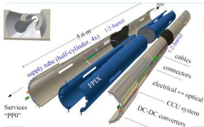
**Figure 3:** Picture of the supply tube mechanics situated on the two sides of the detector barrel. The supply tube holds the control electronics (CCU system and electrical-optical converters.)
