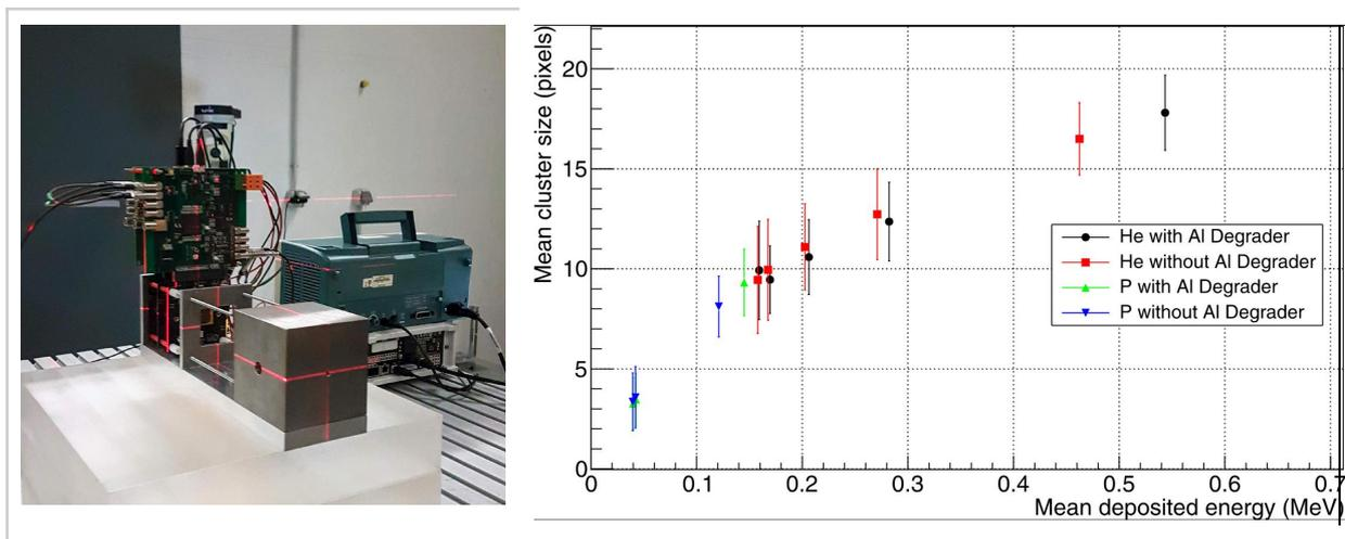
**Figure 4.** Left: Test beam setup for the characterization of detectors to be used as sampling calorimeter for the pCT medical application. Right: Energy dependence of the cluster size of the ALPIDE pixel detector.
